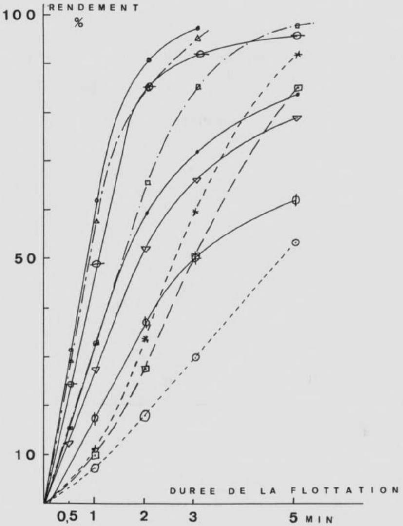
Fig. 1. — Sulfuration de la malachite 270-400 mailles. Influence de la concentration en NaSH.  $\circ$  = 0 mg NaSH/l;  $\nabla$  = 5 mg NaSH/l;  $\bullet$  = 10 mg NaSH/l;  $\circ$  = 20 mg NaSH/l;  $\circ$  = 60 mg NaSH/l;  $\triangle$  = 80 mg NaSH/l;  $\square$  = 90 mg NaSH/l; \* = 100 mg NaSH/l;  $\square$  = 110 mg NaSH/l;  $\circ$  = 150 mg NaSH/l.
