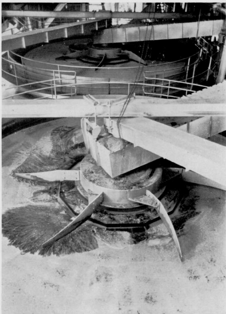
Fig. 4. — Primary I.H.C. — Cleaveland jigs of 25' diameter on Selangor N o 2 dredge (note skimmer with blades).
