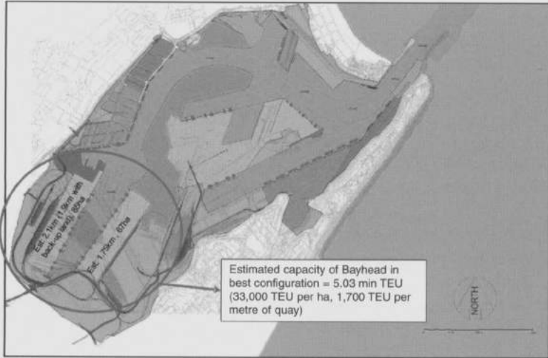
Fig. 4. — Proposal for the Bayhead terminal development in the port of Durban (Source: Transnet).
